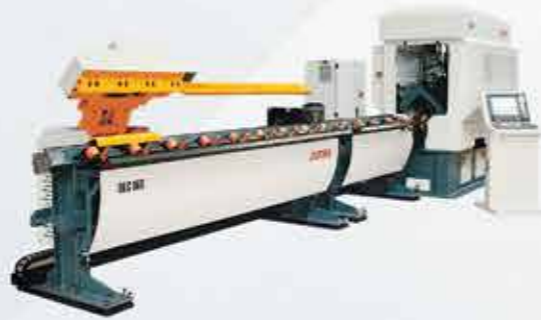
L ANGLE PROCESSING CENTER
