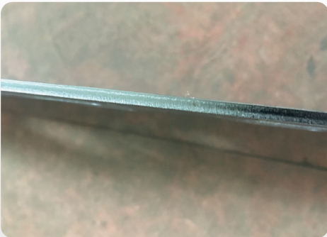
Purity : %99,999 Laser Power : 4 kW Material : 6mm Steel
