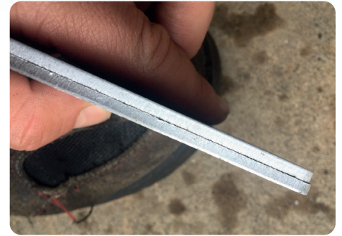
Purity : %99,999 Laser Power : 4 kW Material : 6mm Steel
