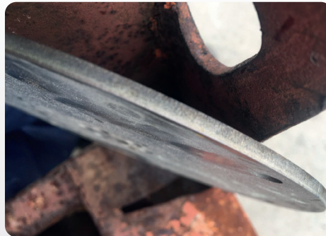
Purity : %99,999 Laser Power : 4 kW Material : 6mm Steel
