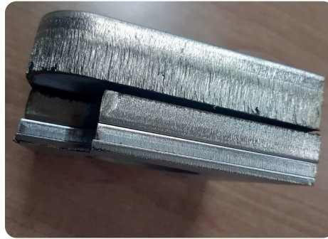
Purity : %99,999 Laser Power : 6 kW Material : 20mm Stainless
