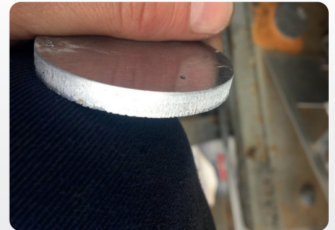
Purity : %99,999 Laser Power : 4 kW Material : 6mm Stainless
