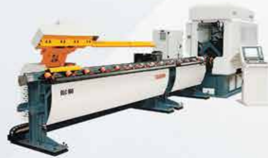
L ANGLE PROCESSING CENTER
