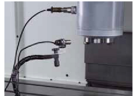
/ Dynamic Vibration Inspection
