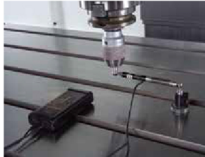
/ High precision ball bar circle inspection.
