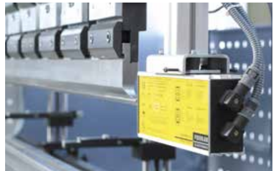
CE Laser Safety System
