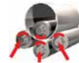
HRB-4R LINEER MERDANE SYSTEMI Üst Top: Ø 460-Ø760 mm Tahrik : Tüm Toplar
